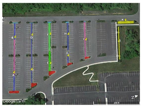
Figure 8: HCC micro-bioretention swales A-K color coded for planting scheme. See Planting Legend for details.
